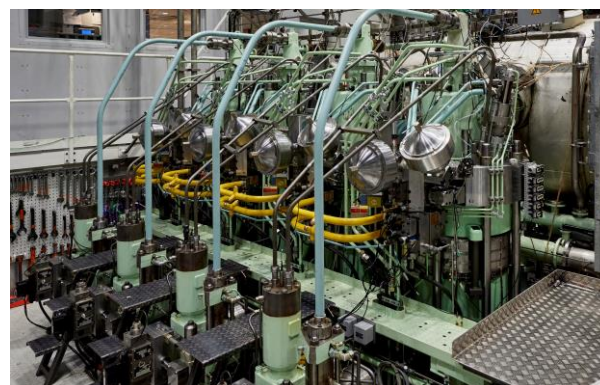
Figure 14. Photo of MAN B&W 4T50ME-X rebuilt to full engine operation on ammonia.
