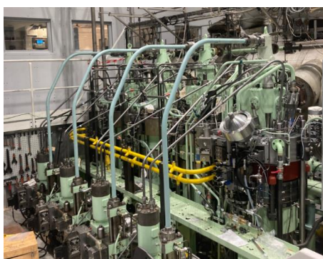
Figure 1. Photo of cylinder cover for ammonia tests mounted on the MAN B&W 4T50ME-X test engine in Copenhagen.
