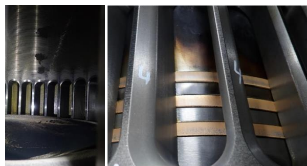
Figure 13. Photos from cylinder inspection of the \text{NH}_3 test cylinder.
