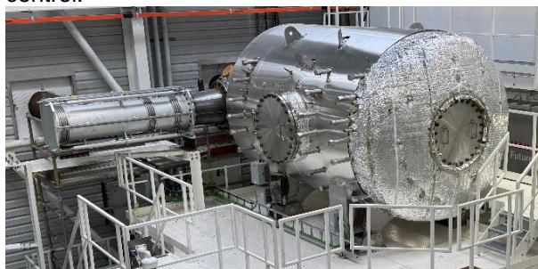
Figure 15. SCR for 4T50ME-X full engine testing.
