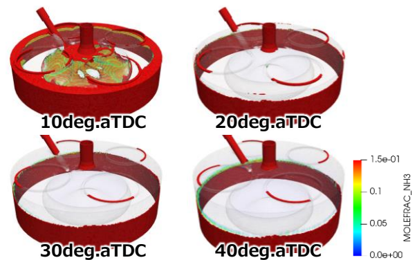
Figure 15. Unburned NH_3 distribution estimated by 3D-CFD simulation at GFER = 95\%
