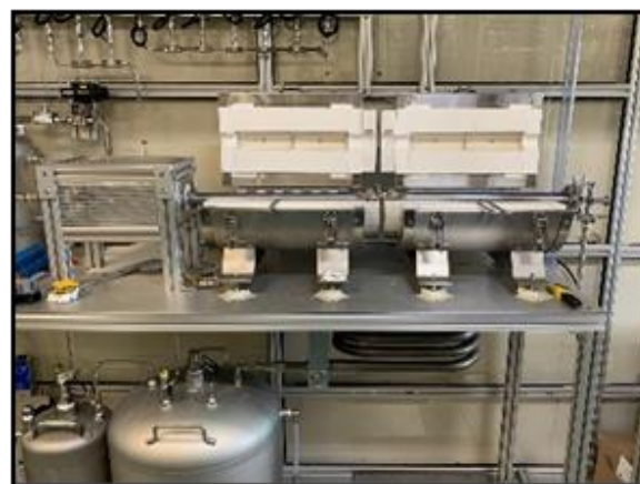
Figure 14 – Test rig for chromium poisoning
