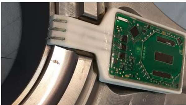
Figure 27. Picture of the Miba telemetric system with 3 thermocouples mounted on a HiPo engine connecting rod
