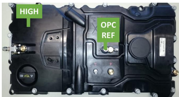
Figure 2. Valve cover with ports for extracting aerosol “OPC REF” and adding purge air “HIGH”.
