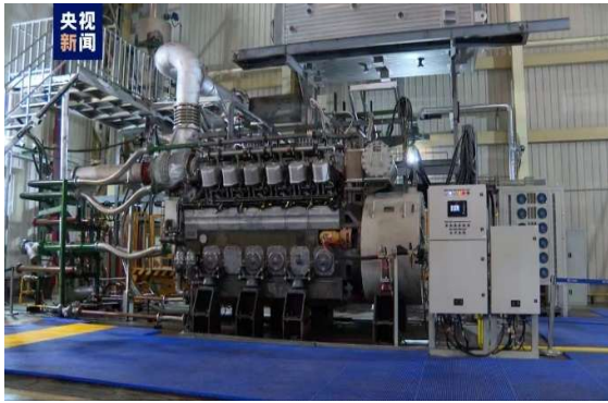
Figure 5. R&D test cell for the new ammonia dual-fuel engine 12V240H-DFA
