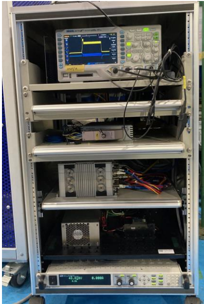
Figure8. Customized RCP for a single cylinder engine test bench (dSPACE Micro Autobox II + Rapid PRO)
