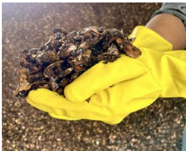
Figure 1. Cashew nut shell presscake after extraction of cashew nut shell liquid as feedstock for the production of pyrolysis oil and biochar.
