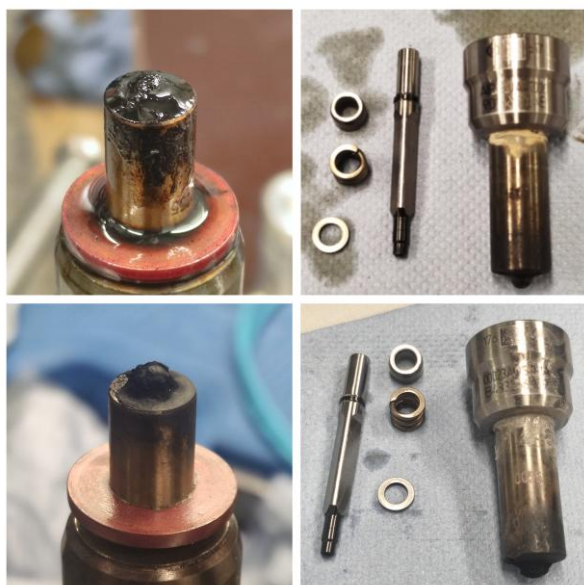
Figure 8. Deposit formation on fuel injection nozzle tip and on injector needle after running on B20 MASH POCC/VLSFO blend (top) and after running on problematic biofuel-blend (bottom). [13]
