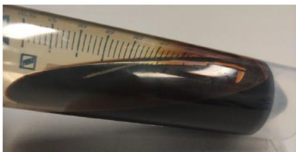
Figure 3. Compatibility/mixing stability of B20 POCC/VLSFO blend with diesel fuel.
