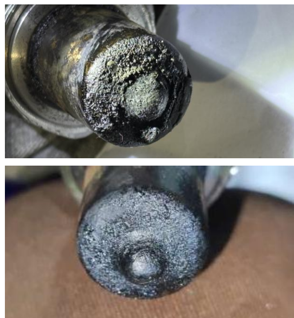
Figure 14. Deposit build-up on the fuel injection nozzle after 60 operating hours (top) and after 360 operating hours (bottom).
