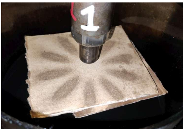
Figure 15. Spray pattern at 400 bar nominal opening pressure in an injector calibration rig after 250 operating hours.
