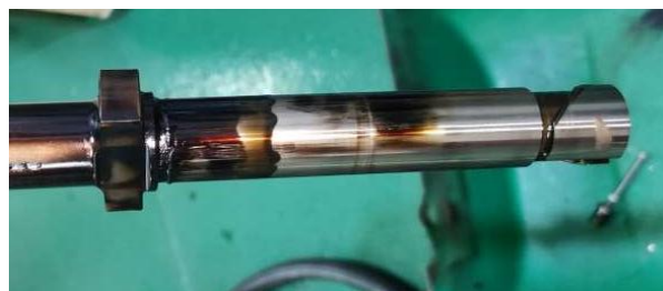
Figure 17. Plunger of a fuel injection pump after 360 operating hours.
