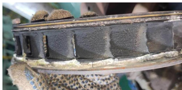
Figure 18. Deposit build-up on turbine nozzle ring after 360 operating hours.
