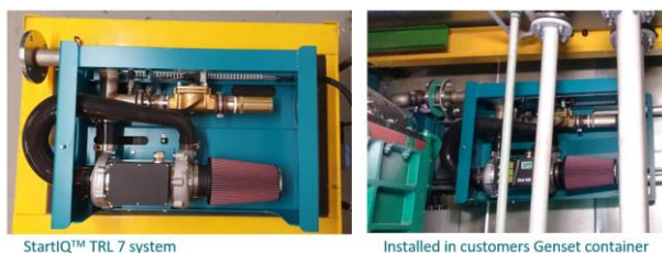
Figure 19. TRL 7 eCompressor system installation in Genset container.
