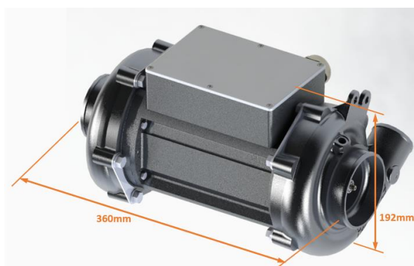
Figure 5. StartIQ™ eCompressor: 55kW, 90krpm, 12.05kg, 192mm height, 360mm length
